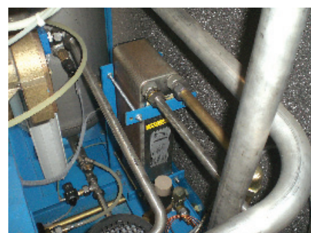
Integrated heat recovery with plate-type heat exchanger
