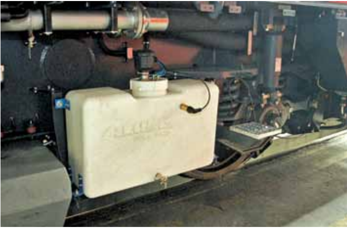
Any condensate produced is collected in a 70 l receiver
