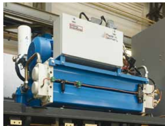
The adsorption dryer in the solution implemented for Stadler is installed horizontally
