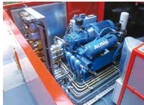
The Track-Air screw compressors are supplied as a complete package with a drive, dryer, controls, condensate receiver etc.
